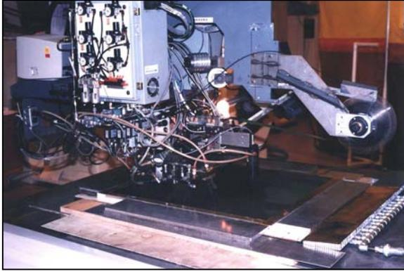
core precoated with BRx-5 paste adhesive and FMx-5 film adhesive. Secondly bonded facesheets were bonded with BRx-5 past adhesive under light autoclave pressure. Figure 8.1 shows the Cytac Engineered Materials in situ consolidation head placing a laminate directly over titanium core. Run on and run off tooling surrounds the core so it cannot be easily seen in the photograph.
