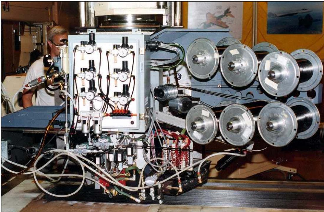
Figure 6.2 Deposition head in situ consolidating 12 thermoplastic tows.
