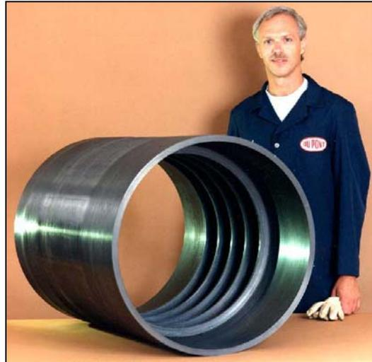
Figure 2.1 The APC-2/AS-4 ring-stiffened cylinder had a  $[90^{\circ}_{2.27}/0^{\circ}]_n$  laminate stacking sequence and five integral 90° ring stiffeners.
